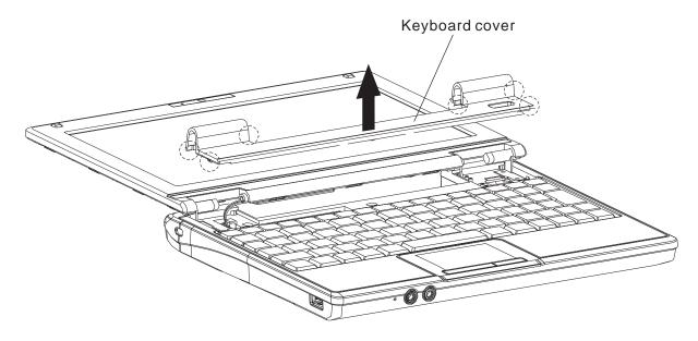
Figure 4-5 Removing the keyboard cover and keyboard
